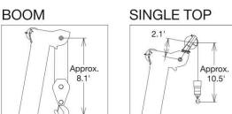
NOTE: Boom geometry shown are for unloaded condition and machine standing level on firm supporting surface.
